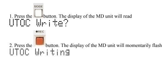
After completing the writing of the "User Table of Contents" (or UTOC) the unit will return to the ready mode for further recording or playback.
